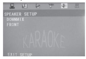
Unload disc, press SETUP KEY to open the SETUP MENU, then press Direction KEY [◀/▶] to select SPEAKER SETUP. The SUB-MENU contains:
